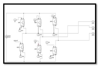
Figure 2: Three Phase Inverter Circuit
