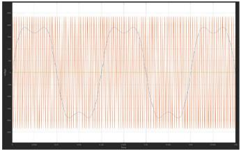
Figure 4: Simulation results obtained for three-phase modulating waveform and phase shifted carrier wave
