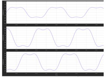
Figure 5 : Simulation results for three phase  $3^{rd}$  harmonic + sine wave
